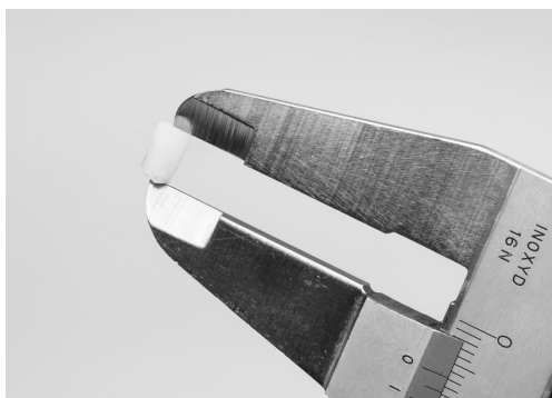
Figure 86 – Measuring the depth of the test plug
