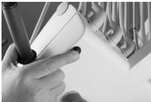
Figure 38 – Initiating selection of instrument to be used with XO Peristaltic Pump
