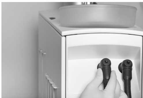
Figure 77 – Removal of suction hoses and filters
