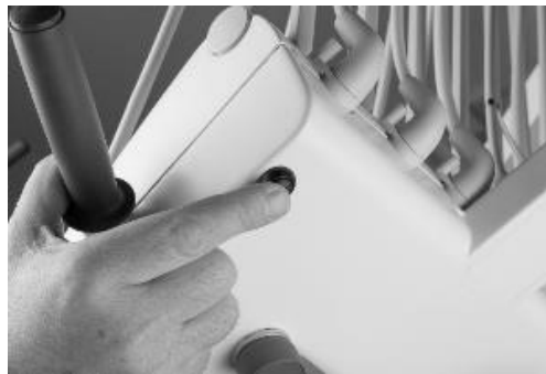
Figure 65 – Configuration button (1) under the instrument bridge
