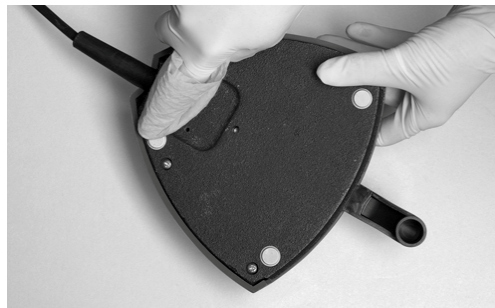
Figure 82 – Cleaning of foot control “rubber feet”
