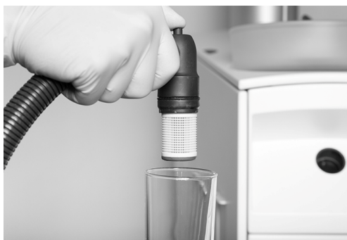
Figure 78 – Press the button to eject the filter
