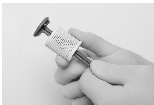
Figure 79 – Removing filter cartridge from filter holder
