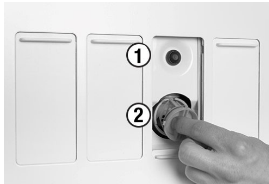
Figure 89 – Manual activation of cuspidor valve (1) and cuspidor valve filter (2)
