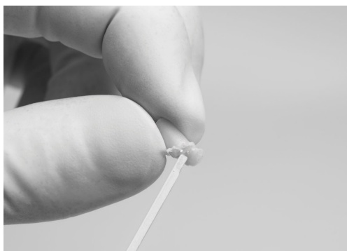
Figure 85 – Non-polymerized material is removed from composite test plug
