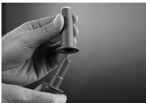
Figure 75 – Removal of suction nozzle covers
