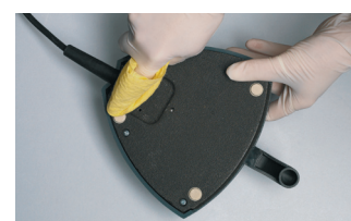
Clean rubber feet under XO Foot Control regularly with benzene.
