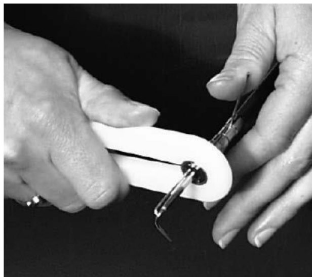
Figure 12 Exchange of ferrite rod
