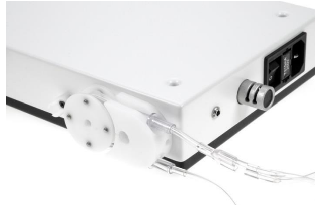
Figure 7 Tubing placed correct around the pump wheel
